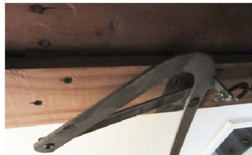
*This hinge arm is bent, which causes rubbing between the parts and excess stress on the hinge. The arms can be bent in such a way that the stairs cannot be easily opened or closed. This damage can cause failure of the stairs.*
